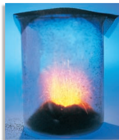
FIGURE 1 The decomposition of ammonium dichromate proceeds rapidly, releasing energy in the form of light and heat.
