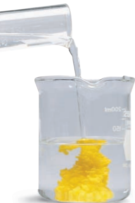
FIGURE 12 The double-displacement reaction between aqueous lead(II) nitrate, \text{Pb}(\text{NO}_3)_2(aq) , and aqueous potassium iodide, \text{KI}(aq) , yields the precipitate lead(II) iodide, \text{PbI}_2(s) .
