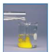
b When solutions of sodium sulfide and cadmium nitrate are mixed, cadmium sulfide, a solid precipitate, forms.
